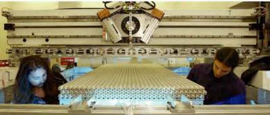
Muon chambers for the outer layers of ATLAS undergo quality control checks (left)
